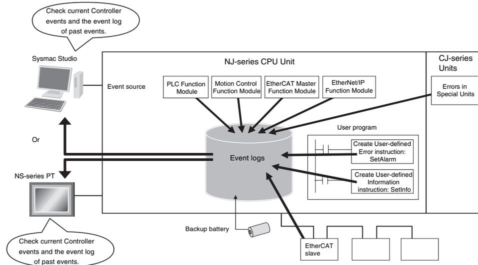
To use an NS-series PT to check events, connect the PT to the built-in EtherNet/IP port on the CPU Unit.
