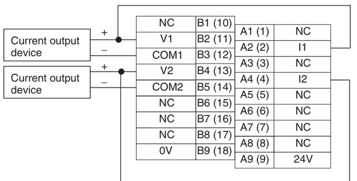
\* Always short-circuit the V and I terminals with the provided short-circuit fitting when using current input.
