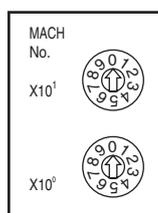
The unit number switch on the front panel of the Unit is used to set the words in the CIO and DM Areas allocated to the Analog I/O Unit.
