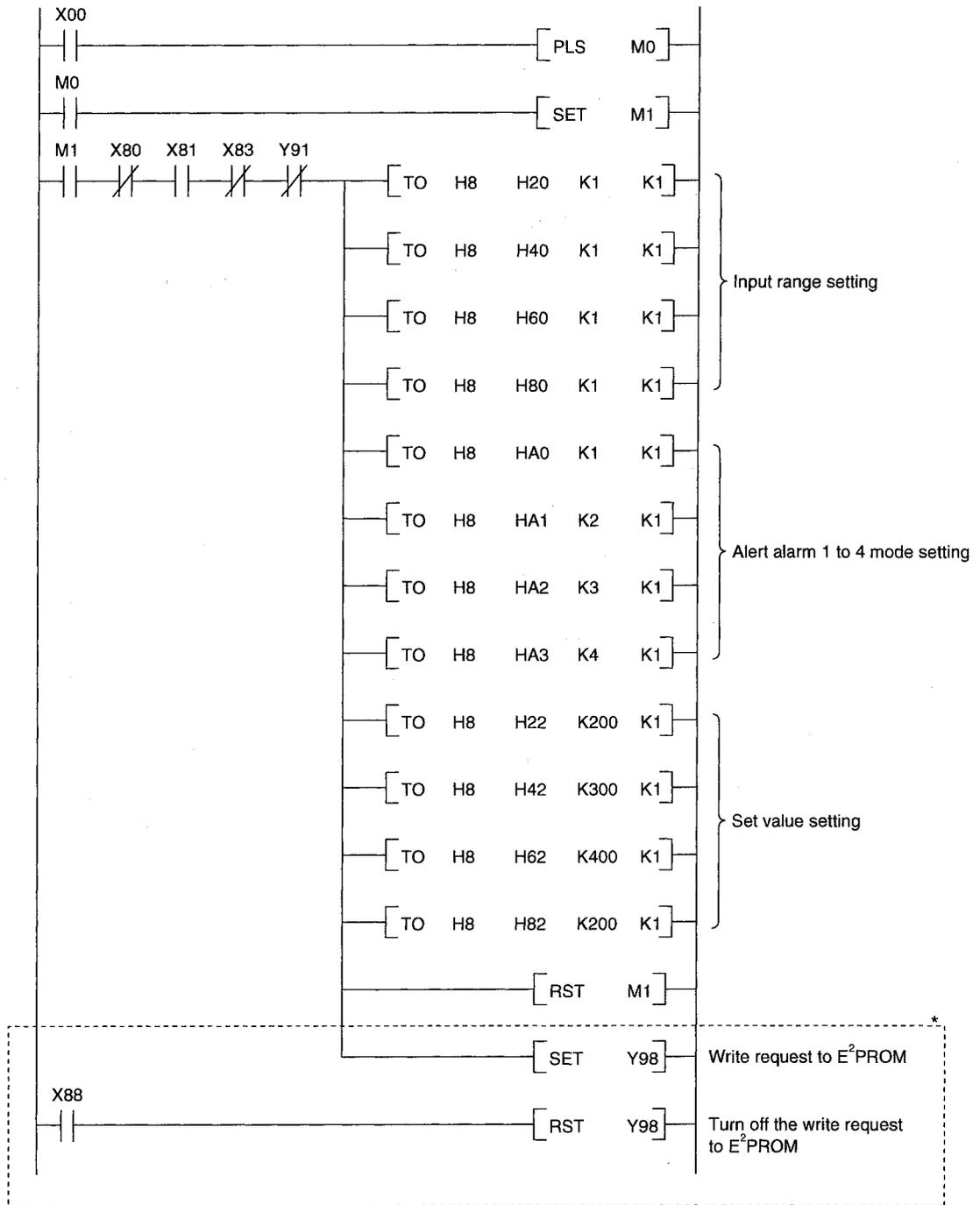
\*: Necessary to register the set input range, alert setting, and set value to the E<sup>2</sup>PROM. When writing the input range, alert setting, or set value using the sequence program during power startup, it is not necessary to write to the E<sup>2</sup>PROM.
