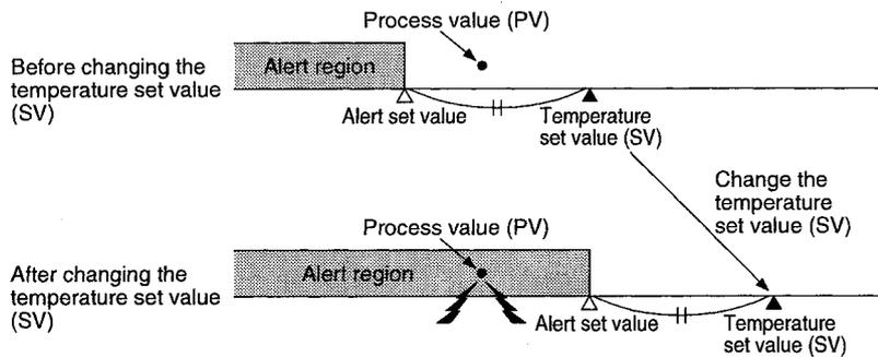
(3) The A1S64TC allows selections for four alarms (alert alarm 1 to 4) from the alert alarm, alert alarm with wait, and alert alarm with re-wait.
