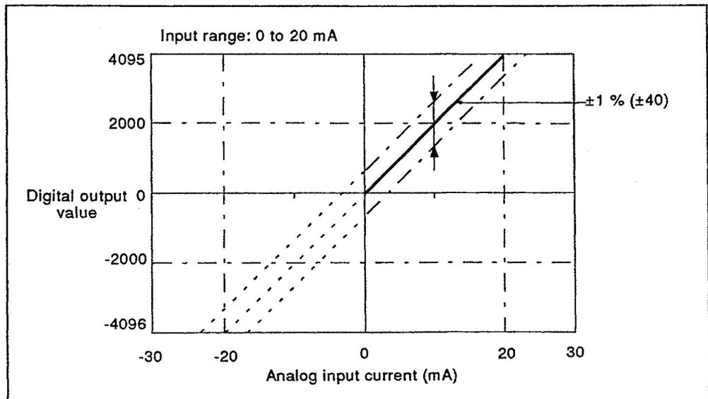
Fig 3.4 Overall Accuracy of the Current Input Characteristics
