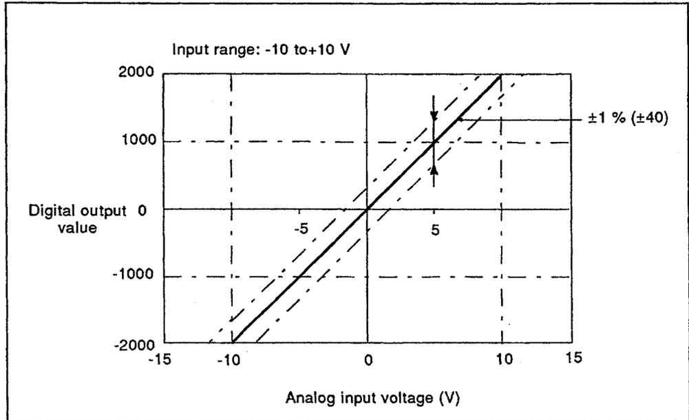
Fig 3.3 Overall Accuracy of the Voltage Input Characteristics
